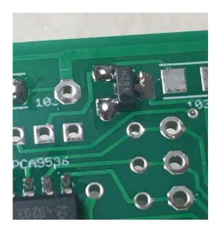
\_ Mount the 10K resistor (marked "103")
