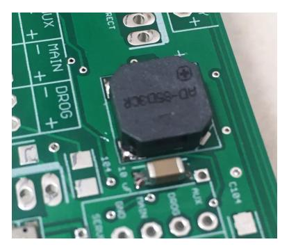
\_\_\_\_\_ Mount the .1 uF capacitor (unmarked brown parts in PAPER tape)
