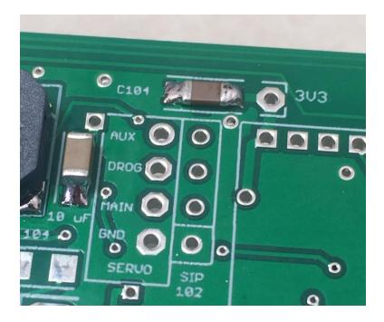
Mount the 100K resistor (marked "104")
