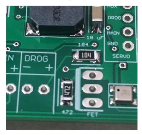
That concludes the surface-mount parts on the top side of the board...
