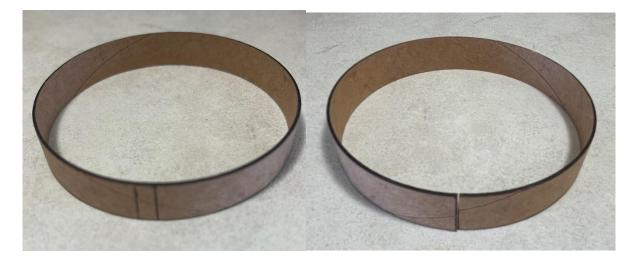
Test-fit the coupler rings inside the coupler, making sure that the rings just fit inside the coupler with the cut ends of the rings just touching. If the ends overlap a bit, trim to fit. It's OK if there is a slight gap, but you do not want the cut ends to overlap.
