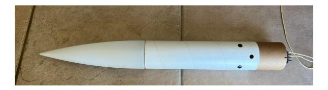
Feed the MAIN shock cord into the main body tube, then carefully attach the AV Bay coupler to the main body tube. The hole for the switch should be centered between two fins, but NOT aligned with the rail buttons (since you're going to need to access it on the pad).
