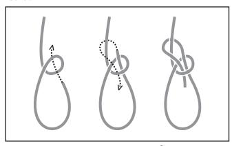
**Step 5.** Tie the yellow **Kevlar** ® **shock cord** through the two holes in the **upper centering ring** using the **Bowline knot.**Tighten the cord and apply a drop of glue to the knot to secure it.
