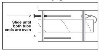
**Step 10.** After the glue dries on the **forward centering ring**, slide off the **rear centering ring** using the **screw head** as a handle.
