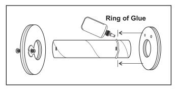
**Step 3.** Apply glue fillets to both sides of the **upper centering ring** joint. Smooth out excess glue with a fingertip.
