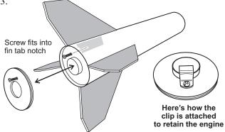
Apply glue to the rear of the **fin tangs** inside the rocket body. Slide the **rear ring** into the body tube until it stops against the glued fin tang edges. Let dry.
