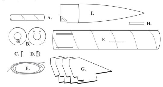
**Step 1.** Locate the **engine mount tube**. With a pencil, mark the tube at 1/4" from the rear edge and 1" down from the forward edge.
