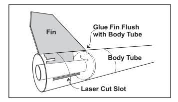
**Step 11.** Place the glued edge of the **fin** in one of the **laser cut slots.** The **fin** tang should contact the engine mount tube and the rear of the fin is flush with the end of the **body tube.**
