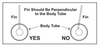
**Step 12.** Hold the **fin** firmly on for at least one minute and do not bump or move it. The **fin** should be perpendicular to the **body tube** as shown below. Hold the **body tube** horizontally with the **fin** sitting up and wait a minute before continuing.
