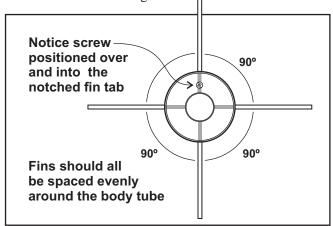
**Step 13.** Repeat Step 11 for the next three **fins.** Allow time between installations so the glue dries well enough to hold the **fins.** When all four **fins** are on correctly, they should look like the diagram above.
