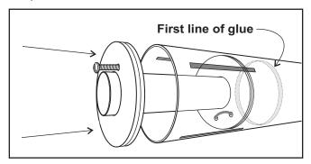
**Step 9.** Push the **engine mount assembly** inside the **body tube** until the **engine mount tube** is even with the end of the **body tube.** Wipe any glue out of the slots. Be sure that the rear **centering ring** is below the slots.
