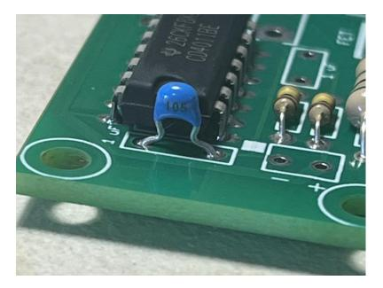
Locate the other 1 uF capacitor, just below and on the right side of the CD4011BE chip. The 1 uF capacitor is marked "105"... make sure you have the right one, there are others that look very similar! Insert it into the board, and use a piece of masking tape to hold it down, then turn the board over and solder the leads to the pads. Clip the leads off close to the board, then remove the masking tape.
