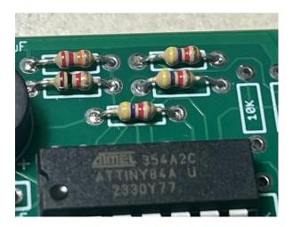
Locate the 4.7K resistor near the bottom of the processor, marked "4.7K". This resistor can be identified by the color bands... yellow-purple-red. Bend the leads close to the body, then insert them into the board. Use a piece of masking tape to hold them down, then turn the board over and solder the leads to the pads. Clip the leads off close to the board, then remove the masking tape.
