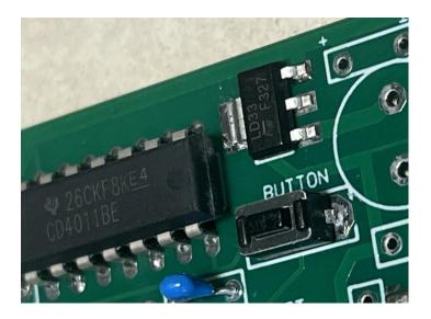
Heat up the large pad with your iron for about 5 seconds or so, then apply solder to the pad and the tab on the regulator. Hold the iron there until the solder is nice and shiny, then withdraw the iron. Let it cool for at least 10 seconds before continuing.
