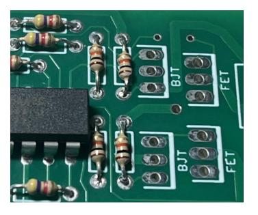
Locate the single 10K resistor next to Pin 1 of the CPU. Bend the leads close to the body, then insert them into the board. Use a piece of masking tape to hold them down, then turn the board over and solder the leads to the pads. Clip the leads off close to the board, then remove the masking tape.
