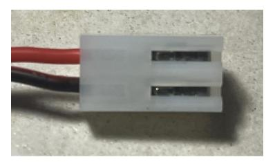
Now, push the socket body into the header on the altimeter, it should lock in place.
