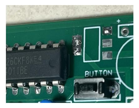
With tweezers, hold the regulator over the pads, then with your soldering iron melt the solder on the top pad. Wait a few seconds for it to completely melt, then withdraw the iron, and hold the regulator in place for another 5 seconds or so. If you let go of the tweezers it should be held in place by that solder joint. Check to see that the regulator is flat on the board... if it is not, reheat the solder joint and try again.
