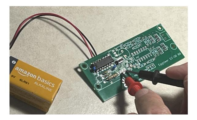
Press the BUTTON and release it. Almost instantly you should see the voltage on those two FET pads jump from 0.0V to 9.0V, or whatever voltage you measured on your battery. It should stay at 9.0V... if it jumps up then goes down to 0.0V, or if it goes to 0.0V as soon as you release the button, you have something soldered incorrectly.
