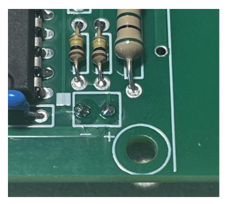
Turn the board over and remove the tape. Check to make SURE that the RED wire is on the "+" pad and the BLACK wire is on the "-" pad. THIS IS CRITICAL... IF YOU HAVE THEM BACKWARDS YOUR BOARD WILL NOT WORK AND YOU MAY DAMAGE SOME COMPONENTS.
