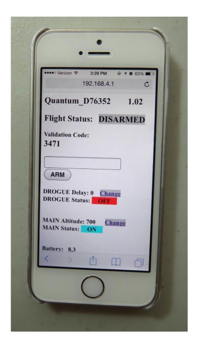
Depending on what you have hooked up to the deployment channels and how it's powered, you may see the deployment channel status displayed in different colors. The colors are:
