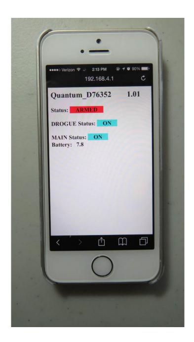
This page looks a lot like the status page, but the status is changed to "ARMED", it doesn't initially have the validation code/box, and only the channel continuity status and the battery voltage are displayed. A few seconds later you should start hearing the buzzer make a rapid "chirping" sound... kind of like a high-pitched warble. This is an audible confirmation that the Quantum is now in flight sequence mode, and you're ready for launch.
