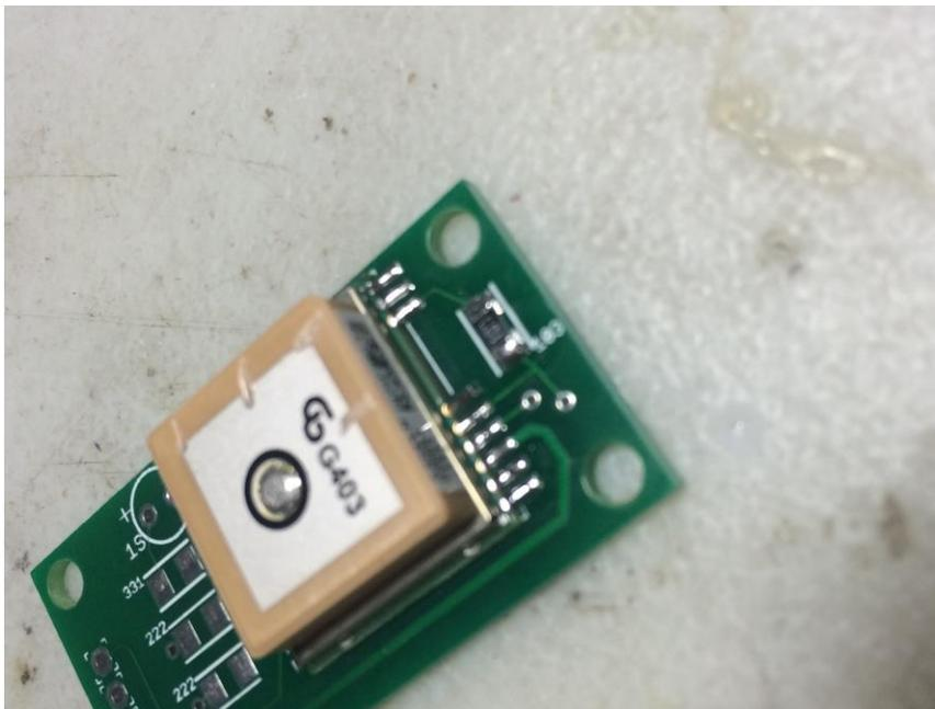
\_\_\_ Mount the 330 ohm Resistor (marked “331” or “3300”)
