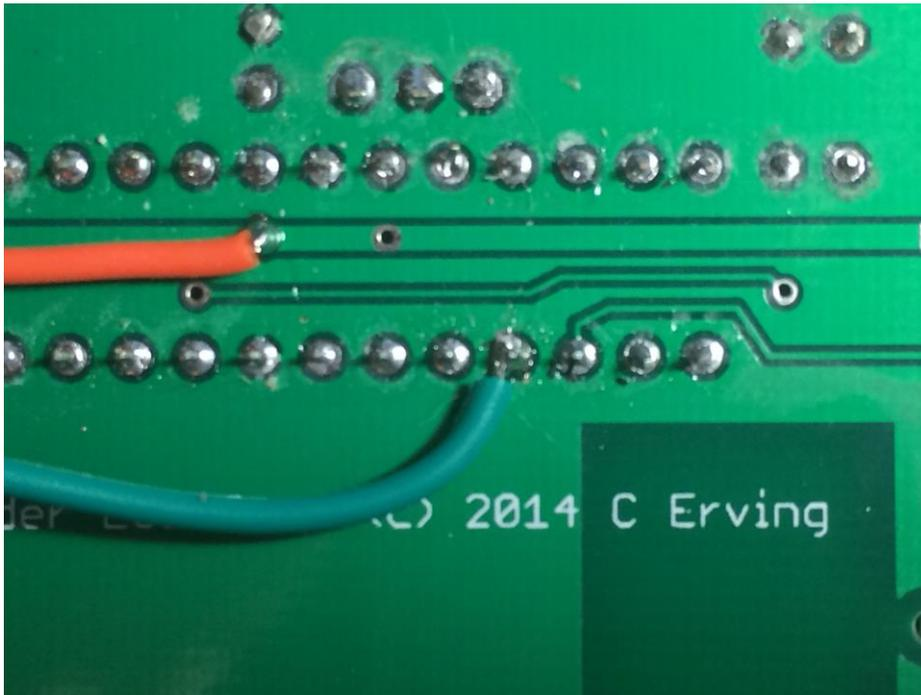
With some paper masking tape, tape the leads down so they can't move. You're done!
