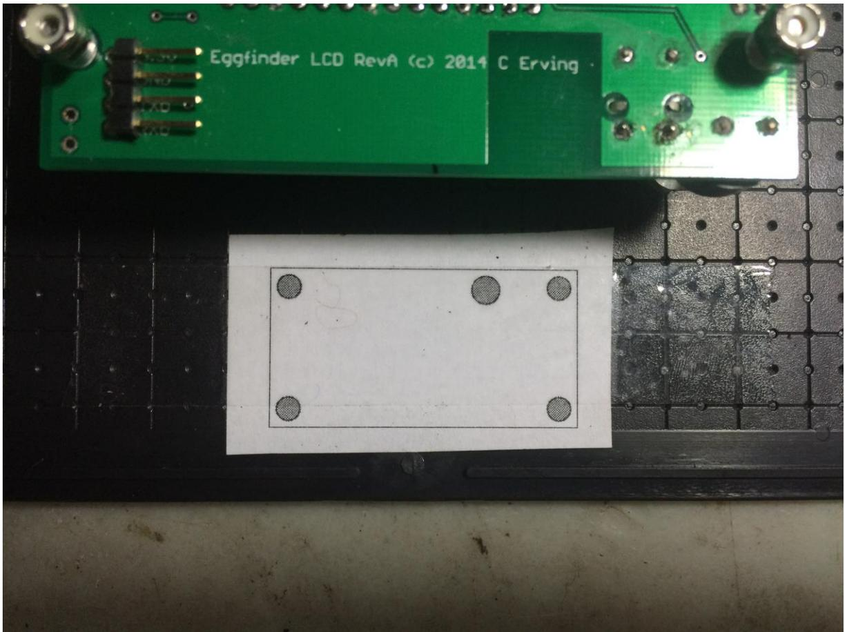
\_\_\_\_ Double-check to make sure that the marks that you made match up with the holes in the PCB board. Remove the LCD-GPS PCB template from the cover, then with a 1/8" drill bit drill the four holes in the corners. Use a 5/32" bit to drill the hole for the LED.
