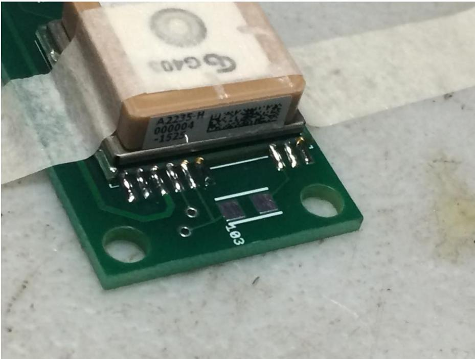
— Remove the masking tape from the GPS module, and remove the masking tape holding the board to your work surface. Turn the module over, and with two new pieces of masking tape tack it down to your work surface so it will not move (yes, it will be upside-down).
