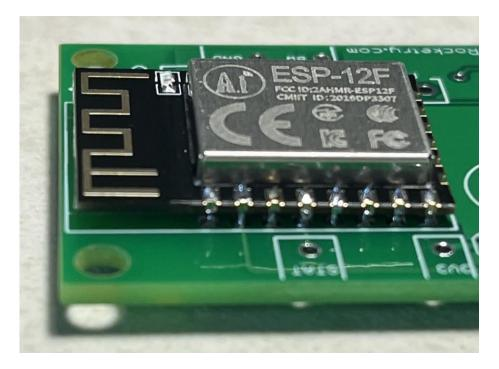
Now, turn the board over so the WiFi module is on the bottom, and solder the leads to the boards. Again, use only enough solder to ensure that you have a good mechanical connection. You may want to clip the leads as you go, making sure that the remnants don't land somewhere on the board.
