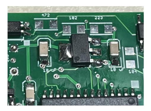
\_\_\_\_ Mount the 4.7K (472) resistor
