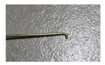
Put the bent end of the antenna into the hole on the top of the board marked ANT, but **do not** solder it in. Tape it down so that it points straight out from the board
