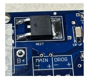
That completes the mounting of the SMT parts on the top of the board. Remove the tape and toothpicks from the board.
