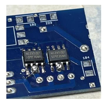
Mount the 100K resistor (marked "104")
