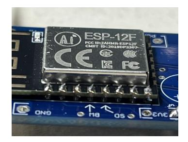
Now, turn the board over so the WiFi module is on the bottom, and solder the leads to the boards. Again, use only enough solder to ensure that you have a good mechanical connection. Clip the leads as you go, making sure that the remnants don't land somewhere on the board.
