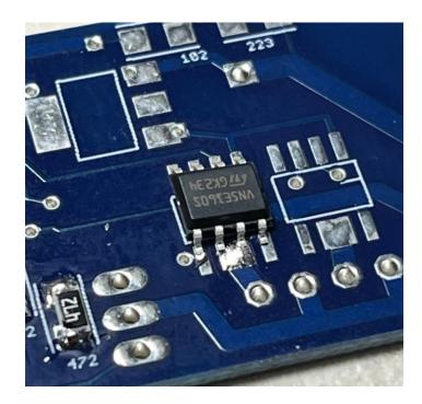
Once you're satisfied with the alignment of the driver chip, solder the remaining leads using the procedure that we detailed earlier. Make sure that you get a good solder joint between the leads and the PC board... it does not take much solder, so do not oversolder them!
