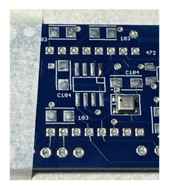
With tweezers, hold the EEPROM in place, and heat the lead over the tinned pad until the solder melts. Keep the heat on for another 3-4 seconds, then remove the iron and let the pad cool.
