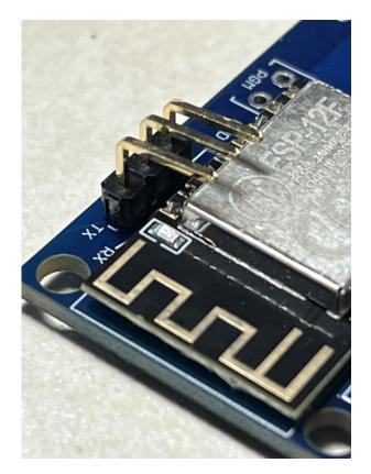
Mount the 3V3 header pin (Optional – for use with the Eggtimer Telemetry Module)
