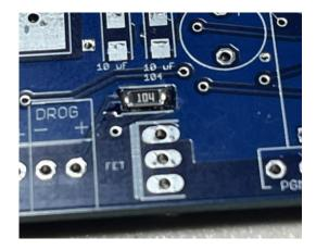
\_\_\_\_ Mount the 10 uF capacitors (unmarked brown parts in CLEAR tape)
