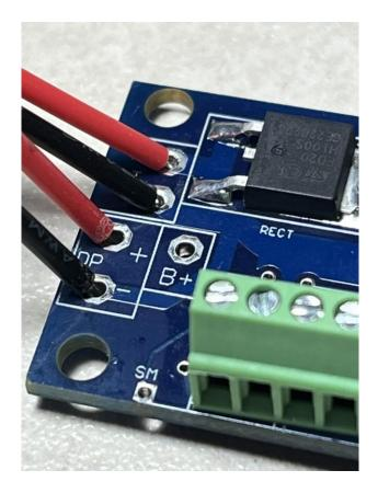
In the picture above, the two power leads on the BAT pads are powering the Quantum's flight computer, and the two power leads on the "DP" pads are powering the deployment outputs.
