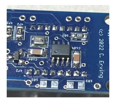
When you are done, all 16 pads (8 on each side) should be soldered on the bottom of the board, and all 16 pads on the WiFi module should be soldered. Inspect the solder joints carefully, and touch up any that look incomplete, particularly the two end pads... they provide the power and ground connections from the board.
