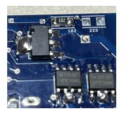
Mount the 22K resistor (marked "223)
