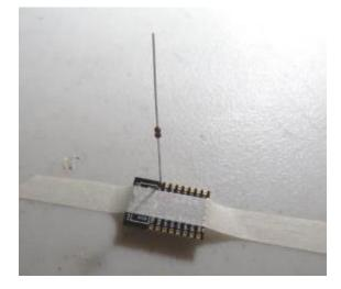
As you clip the resistors' leads, insert it into the next pad, then solder it to that pad. After the second lead on each side, clip it at the resistor body. When you are completely done, there will be a lead on each pad, about  $\frac{1}{2}$ ' long.
