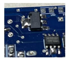
Mount the 1K resistor (marked "102)
