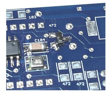
Mount the three 4.7K resistors (marked "472")
