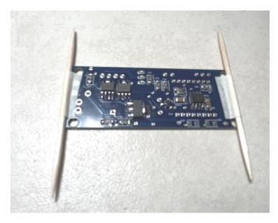
Now, turn the board over and lay it down. The toothpicks should stand the board off from your work surface about 1/8"... this protects the sensitive baro pressure sensor and the other previously bottom-mounted components while you're working on the top of the board.
