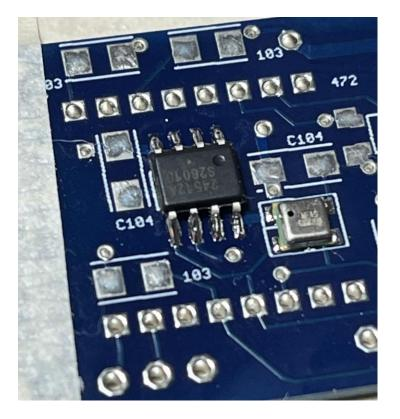
Mount the 10K resistor (marked "103")
