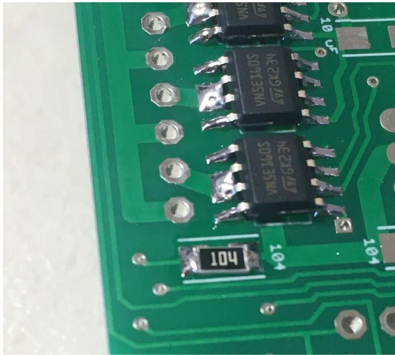
— Mount the 100K resistor (marked “104”)
