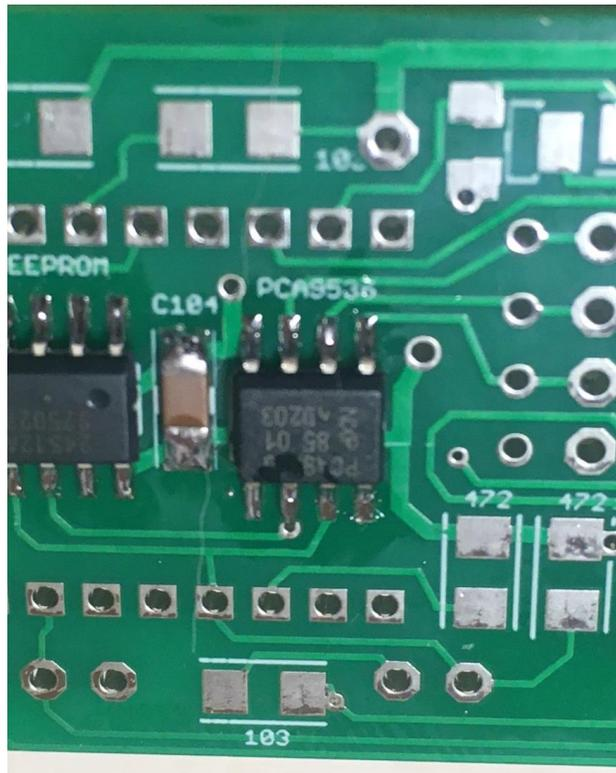
— Mount the 10K resistor (marked “103”)
