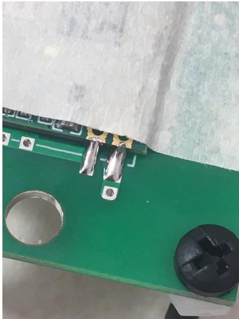
— Inspect all the solder joints on the bottom of the board, using a 10x jeweler's loupe. They should all be nice and shiny, and the solder joints should clearly bridge the parts with the PC board pads. If you have any questionable joints, we recommend that you remove any excess solder with desoldering wick, and resolder.
