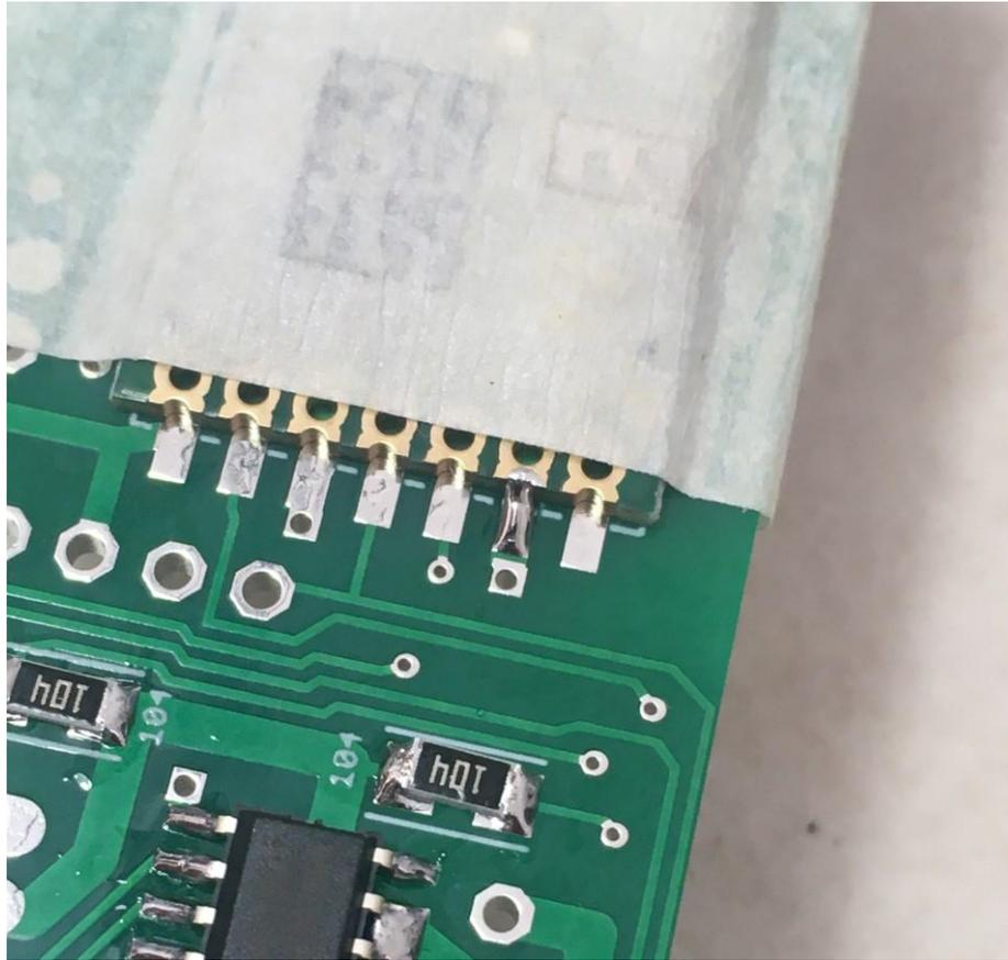
— Check the alignment of the RF module to make sure that the two pads on the other side are centered on the pads. If necessary, heat up the pad that you previously soldered to re-align the module.
