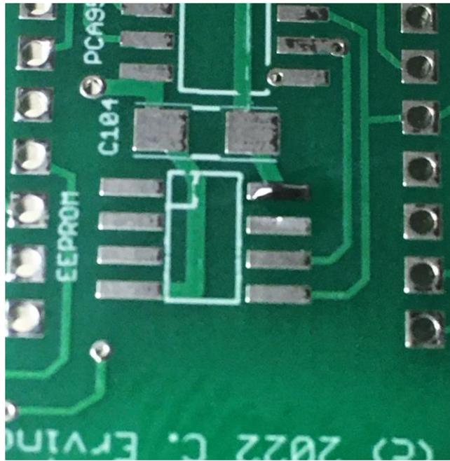
With tweezers, hold the EEPROM in place, and heat the lead over the tinned pad until the solder melts. Keep the heat on for another 3-4 seconds, then remove the iron and let the pad cool. Note that the writing on the chip will appear to be upside-down in relation to the writing on the PC board.
