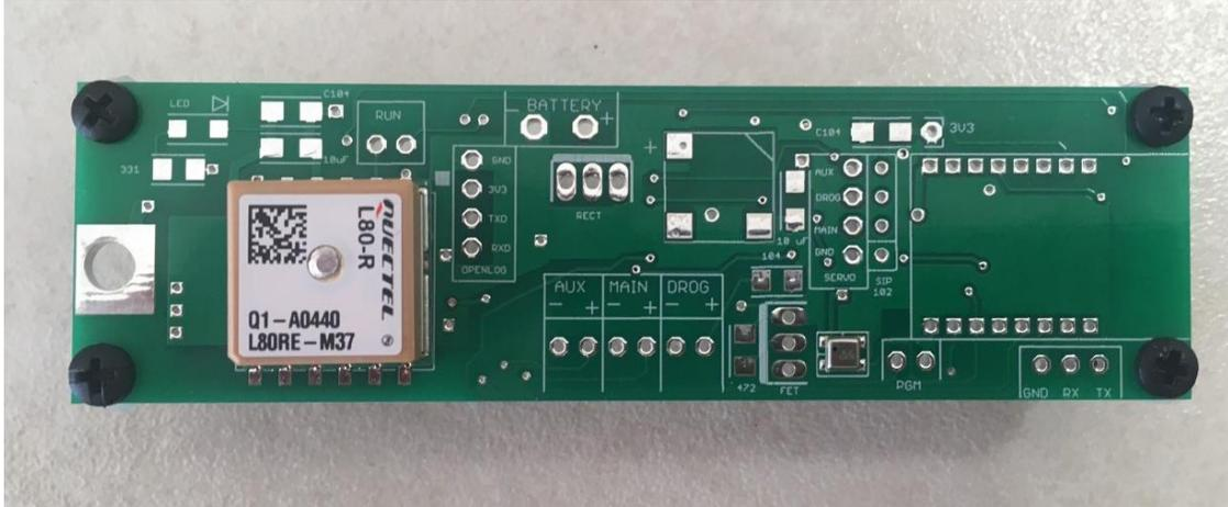
— Mount the 10 uF capacitor (unmarked brown parts in CLEAR tape)
