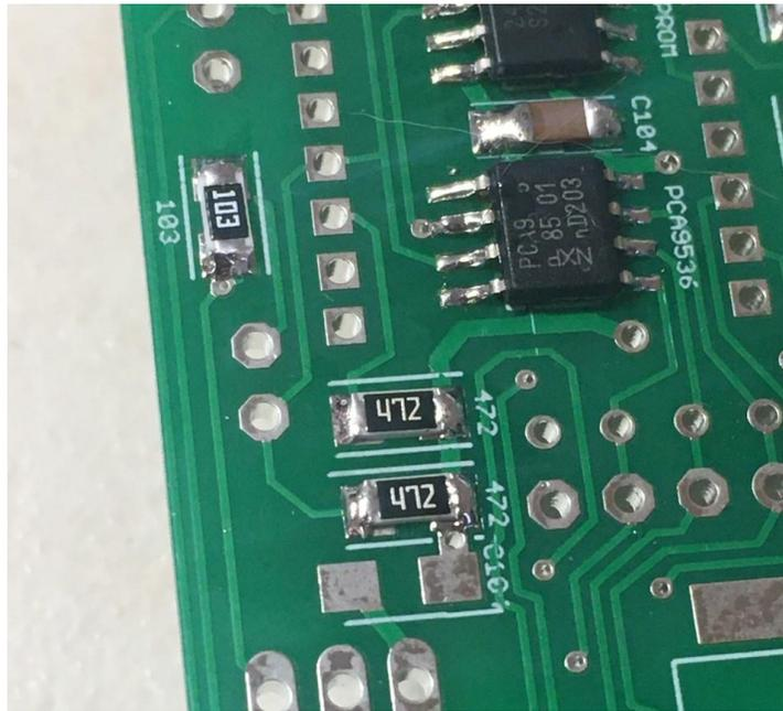
— Mount the .1uF capacitors (unmarked brown part in PAPER carrier)
