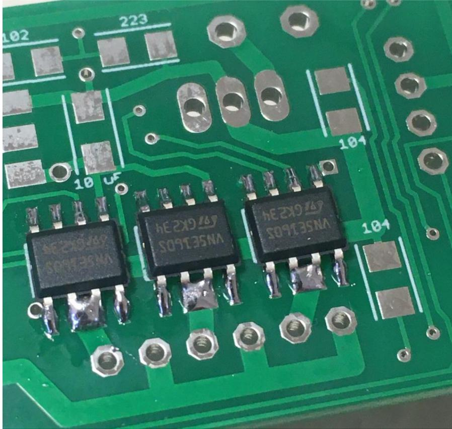
— Mount the 100K resistor (marked “104”)
