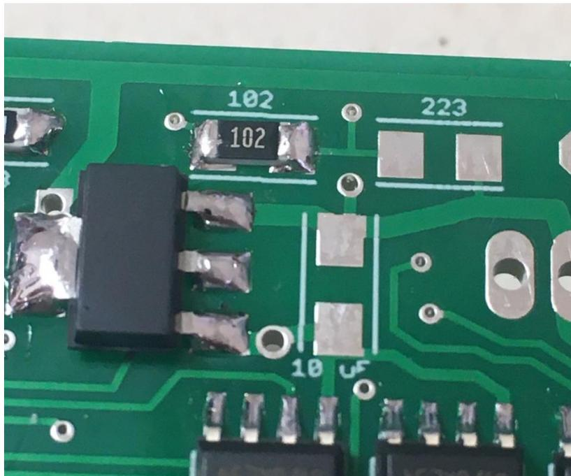
— Mount the 22K resistor (marked “223”)
