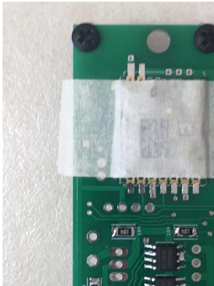
— Solder the second pad from the bottom-right of the Hope RF module to the board. Make sure that the board is properly positioned after you solder this joint; if it moves, heat up the solder joint and move the board slightly so that it is properly positioned. Wait 30 seconds after soldering before continuing.
