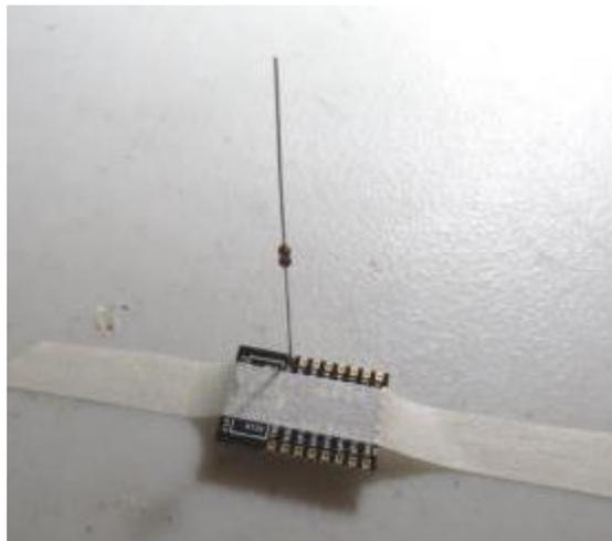
As you clip the resistors’ leads, insert it into the next pad, then solder it to that pad. After the second lead on each side, clip it at the resistor body. When you are completely done, there will be a lead on each pad, about ½” long.
