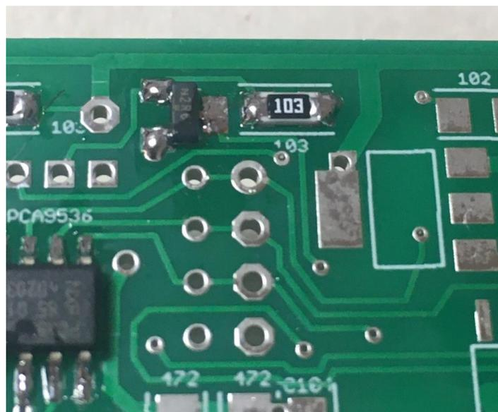
— Mount the two 4.7K resistors (marked “472”)
