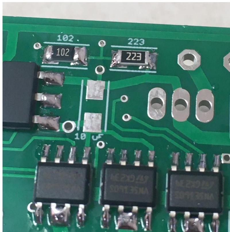
— Mount the 10 uF capacitor (unmarked brown part in CLEAR carrier)
