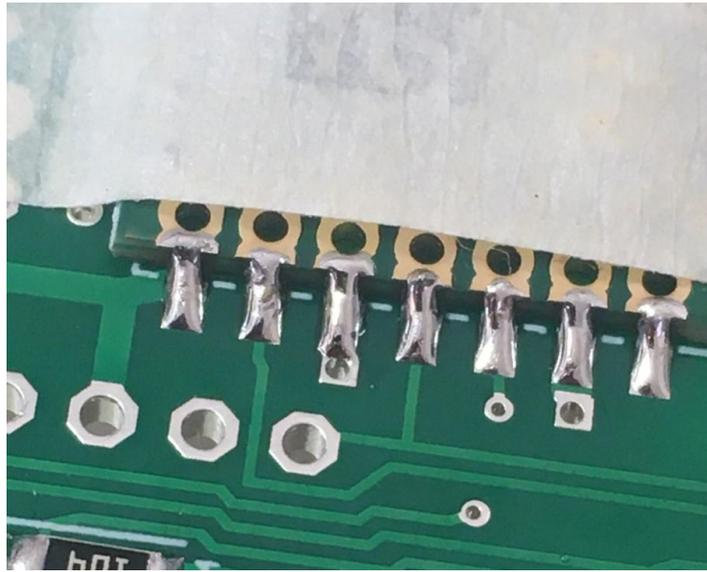
— Turn the board around, and solder the two pads on the other side of the RF module.
