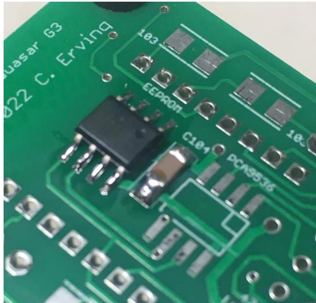
— Mount the PCA9536 I/O Expander (8-pin SOIC chip marked PCA9536)
