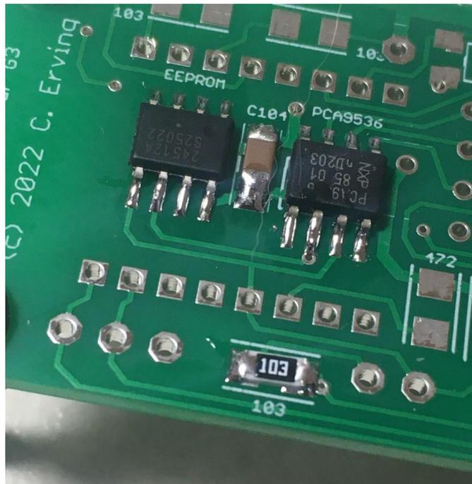
— Mount the two 10K resistors (marked “103”)
