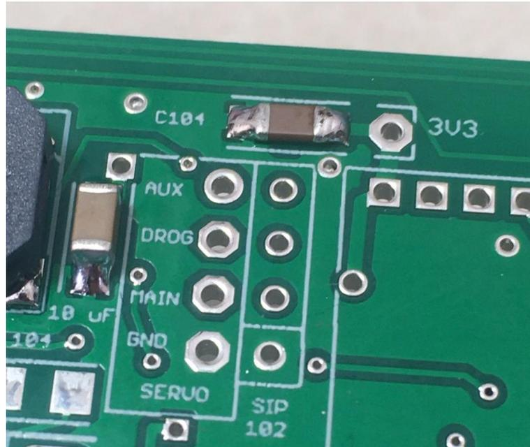
— Mount the 100K resistor (marked "104")
