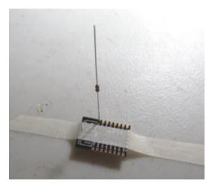
As you clip the resistors' leads, insert it into the next pad, then solder it to that pad. After the second lead on each side, clip it at the resistor body. When you are completely done, there will be a lead on each pad, about ½" long.
