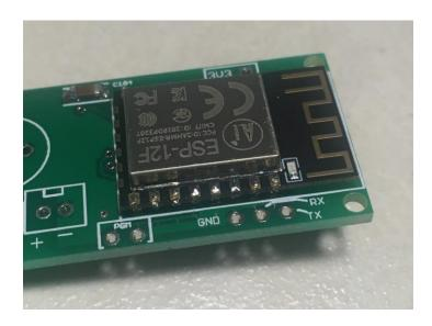
Now, turn the board over, and solder the leads to the bottom side of the board. Again, use only enough solder to ensure that you have a good mechanical connection. Clip the leads as you go, making sure that the remnants don't land somewhere on the board.
