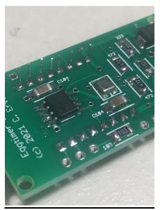
Only one side clipped, for clarity... Be sure to clip the leads on both sides!
