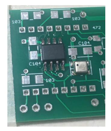
\_\_\_\_ Mount the 10K resistor (marked "103")
