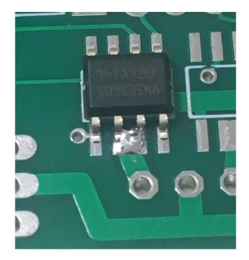
Once you're satisfied with the alignment of the driver chip, solder the remaining leads using the procedure that we detailed earlier. Make sure that you get a good solder joint between the leads and the PC board... it does not take much solder, so do not oversolder them!
