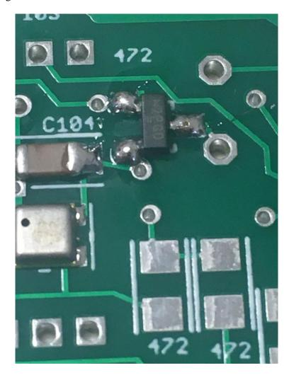
Mount the three 4.7K resistors (marked "472")
