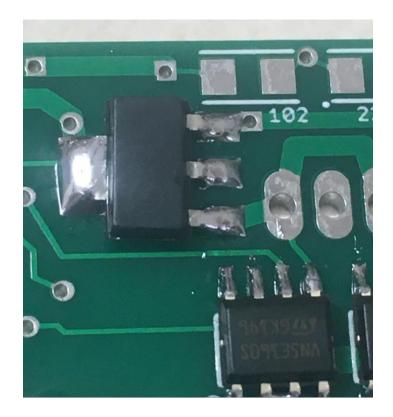
\_\_\_\_ Mount the 1K resistor (marked "102)
