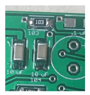
\_ Mount the 0.1 uF capacitor (unmarked brown part in PAPER tape)
