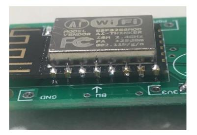
Now, turn the board over so the WiFi module is on the bottom, and solder the leads to the boards. Again, use only enough solder to ensure that you have a good mechanical connection. Clip the leads as you go, making sure that the remnants don't land somewhere on the board.
