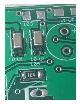
\_\_\_\_ Mount the 10K resistor (marked "103")
