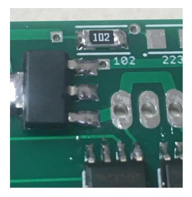
Mount the 22K resistor (marked "223)
