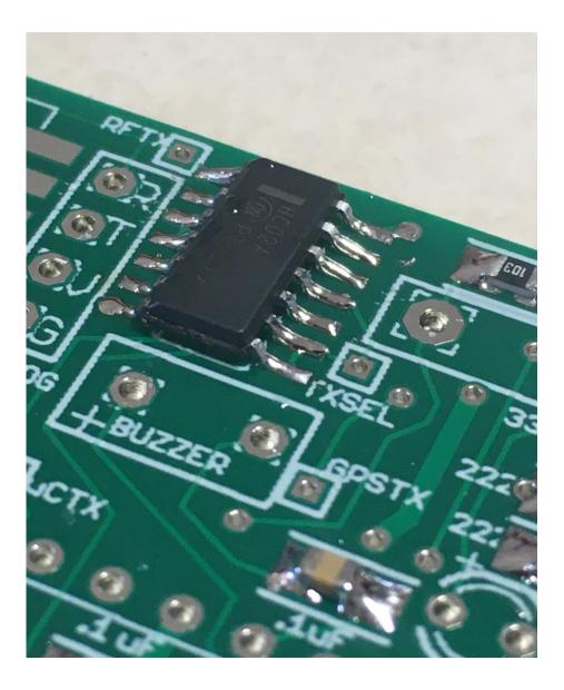
With the 10x jeweler's loupe, inspect all of the solder joints to make sure that they are nice and shiny, cover the pad and the lead, and that there are no bridges. Reheat/resolder as necessary, and use solder wick to clean up any bridges.
