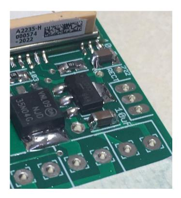
\_\_\_\_ Locate the 22K resistor (marked "223"), it's near the bottom of the board next to the output transistors. Solder it in place.
