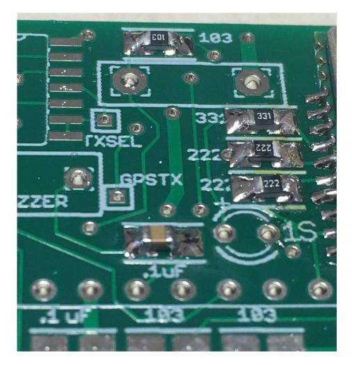
Locate the two 10K resistors between the long row of processor pads, on the right side. Remove two 10K resistors (marked "103") from the tape and solder them in place. Inspect the solder joints with a 10x jeweler's loupe to make sure you don't have any solder bridges.
