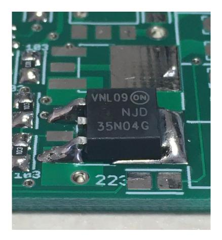
When you are done, inspect the solder joints to make sure that they are nice and shiny and that there are no solder bridges. Note: A solder bridge in an deployment transistor can cause a short that may destroy your Eggtimer TRS, and possibly your LiPo battery too. It may also possibly cause an unexpected deployment when you connect the battery. Be very careful here!
