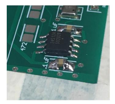
Locate the two 4.7K resistors just above the pressure sensor (it will be marked "472"). Remove two 4.7K resistor (marked "472") from the tape and solder it in place. Inspect the solder joints with a 10x jeweler's loupe to make sure you don't have any solder bridges.
