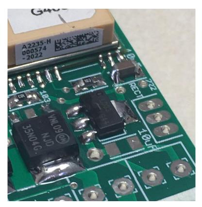
Locate the second 10 uF capacitor just to the left of the pads marked "BATT", it's marked "10 uF". Solder it into place, being careful to avoid solder bridges and inspecting it as you go.
