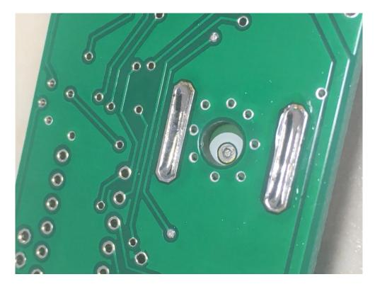
\_\_\_\_ Inspect all GPS module solder joints with a 10x jeweler's loupe to make sure that they are nice and shiny, and that they properly bridge the GPS module pads and the PC board pads.
