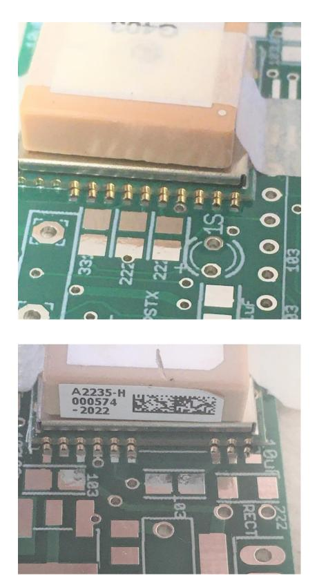
\_\_\_\_\_Using as little solder as possible, solder ONLY one pad in the center of the GPS module. Use only enough solder to get the GPS pad mounted to the board, it won't take very much. You should hold the iron for about 5 seconds after the solder flows, then remove the heat and wait at least 30 seconds before you touch anything. If you do this right, you should see a nice shiny solder joint filling in the gap between the PC board and the GPS module's pad,
