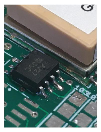
\_\_\_\_ Inspect all of the solder joints with a 10x jeweler's loupe, and redress them as necessary.
