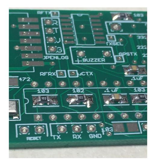
Locate the 10K resistor below the resistors and capacitor that you just soldered, at the bottom edge of the board. Remove ONE 10K resistor (marked "103") from the tape and solder it in place. Inspect the solder joints with a 10x jeweler's loupe to make sure you don't have any solder bridges.
