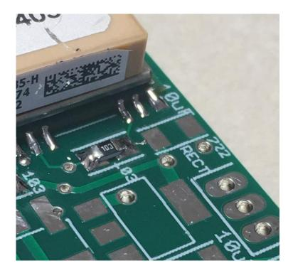
Locate the 10 uF capacitor just to the right of the GPS module near the top, it's marked "10 uF". Solder it into place, being careful to avoid solder bridges and inspecting it as you go.
