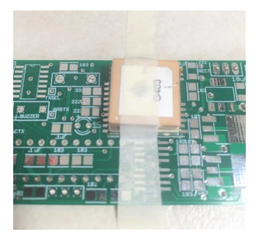
\_\_\_\_\_ DOUBLE-CHECK that the GPS module is properly oriented, and that the pads are centered on the PC board's pads. A jeweler's loupe or small 10x magnifier is very handy for this purpose.
