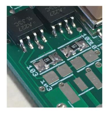
Now, solder three 103 resistors just to the right of the ones that you just soldered.
