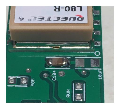
Mount the 10 uF capacitor (brown unmarked part in CLEAR PLASTIC tape)
