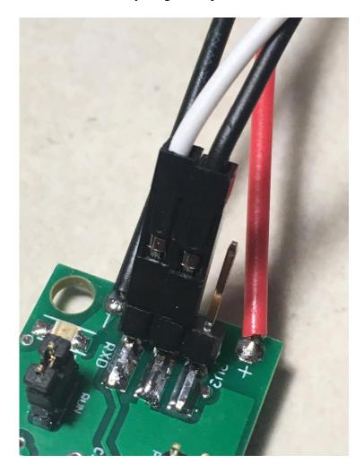
Plug the USB-Serial cable into your computer, and start the terminal program... the settings should be 9600 baud, 8 bits, no stop bits.
