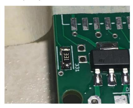
Locate the spot for the 4.7 uF capacitor, it's just to the right of the voltage regulator and is marked "4.7 uF" on the board. Mount it per the procedure above.
