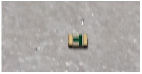
Locate the LED onto the board so that the notch/mark is on the side with the diode marking on the PC board (▶ |). Mount the LED onto the pads, similar to the other parts.
