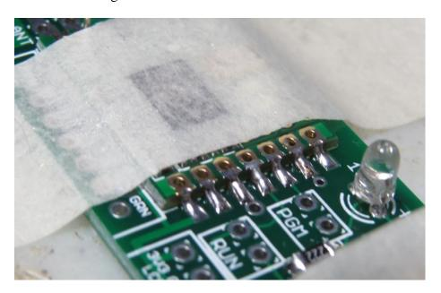
\_\_ If the TX came with a fixed frequency (not 915 MHz), with a permanent marker, write the RF module's frequency on the board in the space provided (i.e. "921"). Since the B and C revisions of the TX board can be frequency-programmed using the Eggfinder LCD you may
