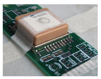
Remove the masking tape from the GPS module, and remove the masking tape holding the board to your work surface. Turn the module over, and with two new pieces of masking tape tack it down to your work surface so it will not move (yes, it will be upside-down).
