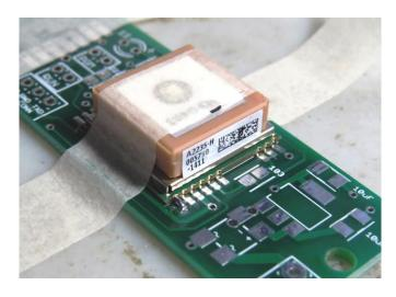
\_\_ CHECK AGAIN that the GPS module is properly oriented and that the pads are centered on the PC board's pads. If the GPS module moved a little during soldering, heat up the solder joint and GENTLY move it into place. If you cannot get it to move without removing it, remove the masking tape, heat up the solder joint, then GENTLY lift the module from the board. Remove the solder with some wick, get a new piece of masking tape, and try again.
