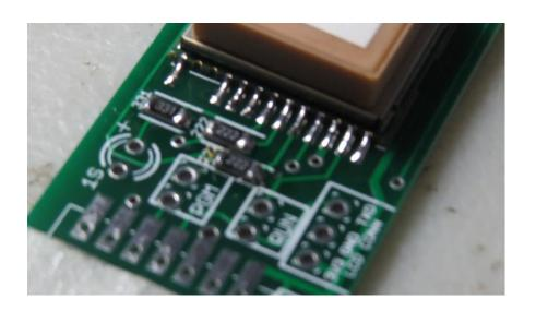
\_\_\_\_ Mount the 10K resistor (marked "103" or "1022")
