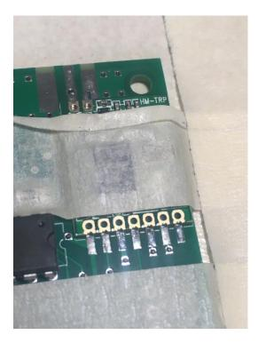
\_\_\_\_\_ Solder the BOTTOM RIGHT pad of the Hope RF module to the board. Make sure that the board is properly positioned after you solder this joint; it it moves, heat up the solder joint
