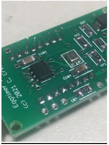
Only one side clipped, for clarity... Be sure to clip the leads on both sides!
