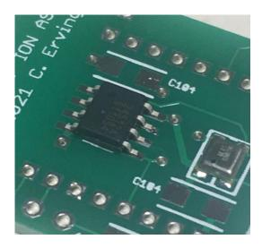
Once you're satisfied with the alignment, carefully solder the remaining leads to the pads, waiting 15 seconds between each lead so that the device has a chance to cool down a bit. We recommend that you do the corners first, to help keep the EEPROM in alignment with the pads. When you're done, get out the 10x jeweler's loupe and inspect each solder joint
