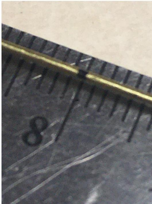
\_\_\_ With a pair of sharp diagonal pliers, cut the wire at the 80mm mark.
