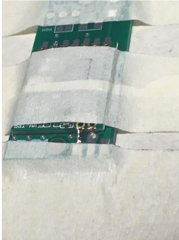
— Solder the remaining six pads on the bottom side of the RF module to the board, waiting 30 seconds between pads to prevent the module from overheating. Do not solder the pad on the other side yet (the side that has only two pads), the one marked “ANT”; you will solder that when you mount the antenna.
