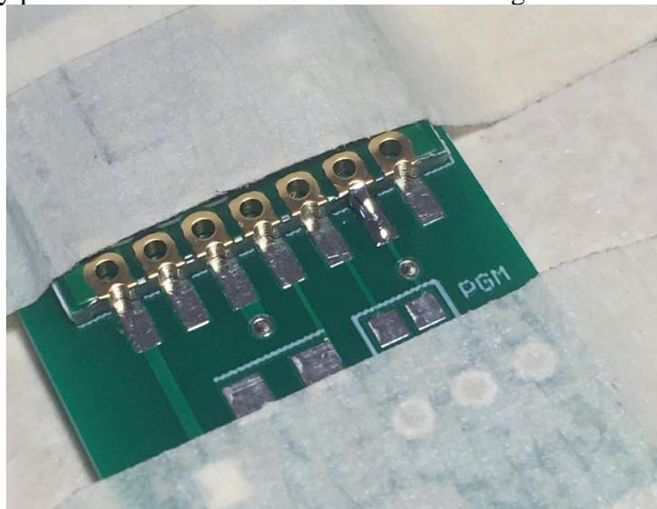
— Check the alignment of the RF module to make sure that the two pads on the other side are centered on the pads. If necessary, heat up the pad that you previously soldered to re-align the module. When you are satisfied with the pad alignment, solder the pad on the left side (the one NOT marked "ANT") to the pad.
