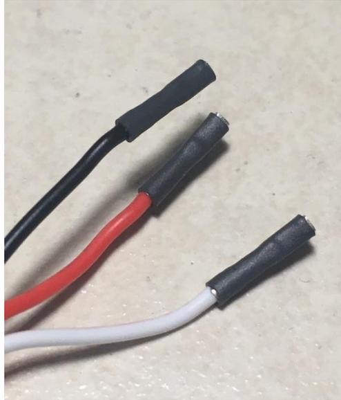
\_\_\_ Insert the tinned wires into the three pads marked "DATA IN", so that the colors match the markings on the PC board: WHITE to "W", RED to "R", and BLACK to "B". With a piece of masking tape, hold the cable in place.
