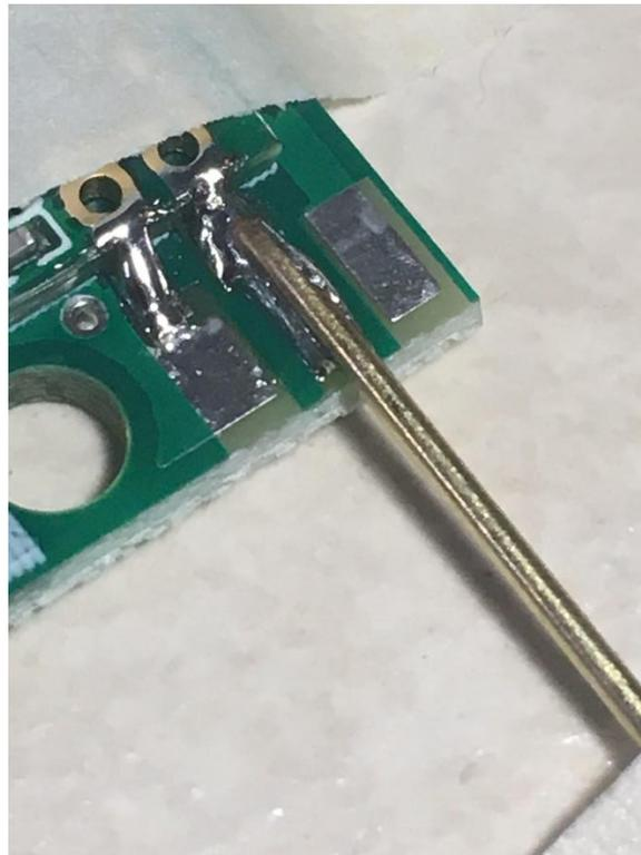
\_\_\_ Measure 80 mm (8.0 cm) from the edge of the board, and mark the antenna wire there.
