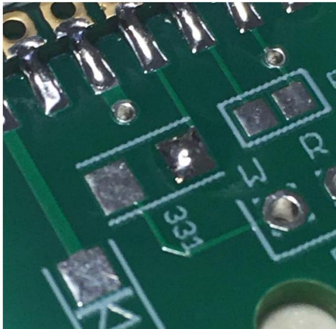
\_\_\_ Heat up the tinned pad, then with tweezers set the resistor onto the pads so that it is centered. Remove the heat, then hold the resistor for about 3-5 seconds so the solder can set.
