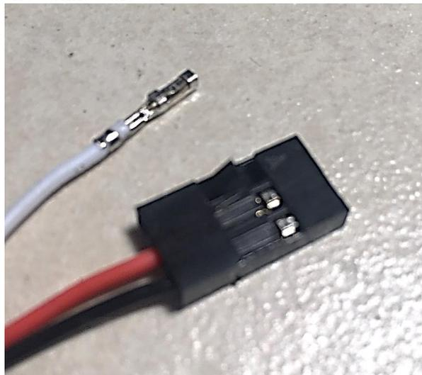
\_\_\_ Repeat for the red and black wires. When you're done, you should have the three wires terminating in socket pins.
