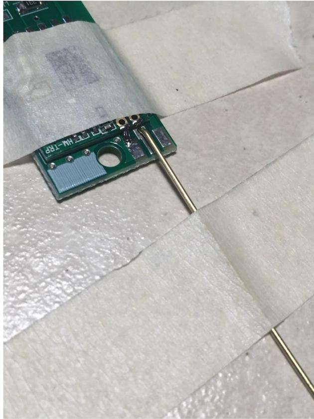
\_\_\_ Solder the antenna to the board, making sure that the solder also extends to the pad on the RF module. A good solder joint should have the antenna connecting to the pad from the hole all the way to the end of the board.
