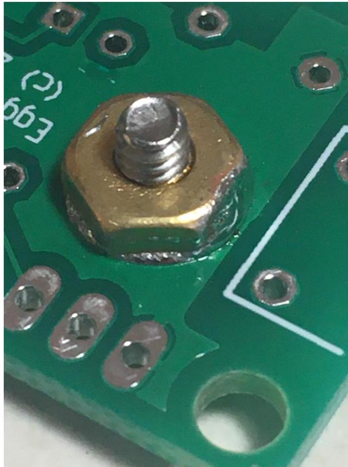
Once you're satisfied with the solder joint, allow the nut to cool for approximately 5 minutes, then turn the board over and back out the screw about two turns.
