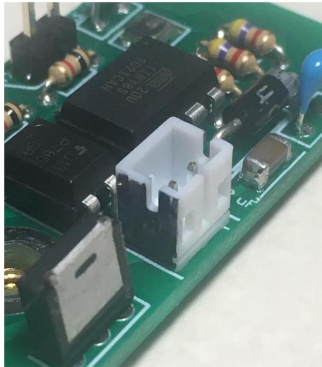
**Battery Connector – Rev D7 Board**
