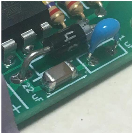
\_\_\_ Go back and reheat the previously-tinned and soldered pad if you don't have a fillet of solder there.
