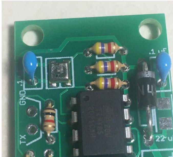
\_\_\_ Locate the spot for the transistor, at the bottom-right of the board. Note that the silkscreen legend has a large “flat” mark at one end, towards the edge of the board... that mark must match the metal tab on the transistor. Note that the position for the transistor is different in the Rev D9 board vs. the Rev D7 board... see the pictures below to identify the location of the transistor.
