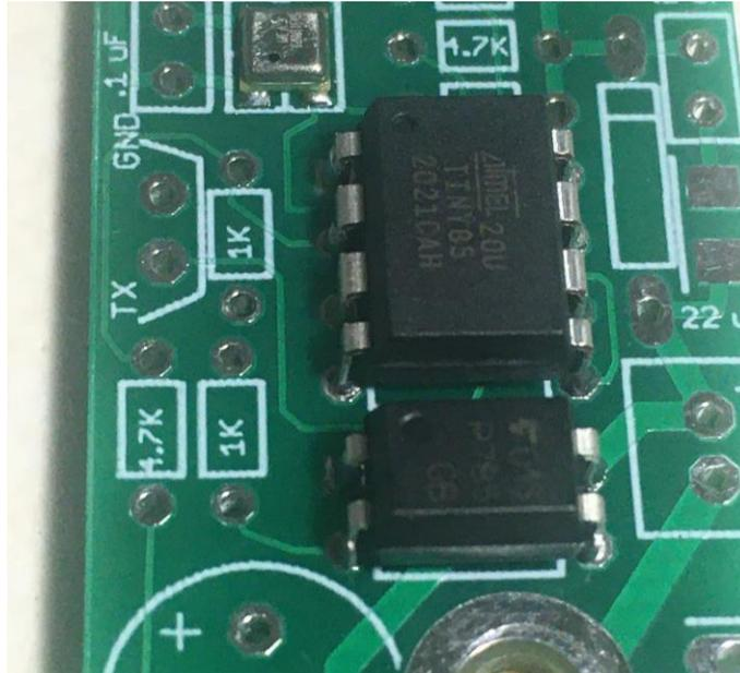
Turn the board over and solder the four pins into the pads. Remove the masking tape.
