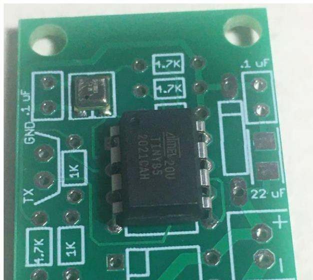
\_\_\_ Locate the spot for the optoisolator, it's the 4-pin part just below the processor. Note that there is a notch marked on the silkscreen, this corresponds to the Pin-1 mark on the optoisolator chip. This MUST match with the "Pin 1" side of the optoisolator. If you look at the optoisolator, you will see an indent, dot, triangle, or bar at one end of the package. That side is the one that must be matched up with the notch on the board.
