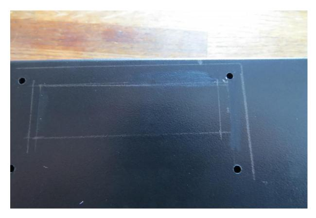
With a 1/8" drill bit, drill out the four mounting holes. Cut a  $\frac{1}{4}$ " sound hole 5/16" below and 1/8" to the right of the bottom-left mounting hole.
