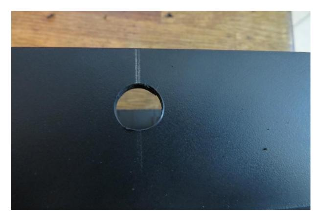
Now you need to drill a hole for the battery box switch. Drill a pilot hole in the bottom of the case bottom, 1" from the left edge and 1" from the bottom edge. Drill it out to ½" with a spade bit.
