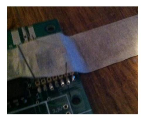
\_\_\_ Stick a round toothpick in the hole in the middle of the solder pad marked ANT. This is to prevent any solder from getting into the hole. Solder the TOP LEFT pad of the Hope RF module to the board, this is the one next to the ANT terminal. Again, DO NOT OVERSOLDER! Wait 30 seconds, then remove the toothpick.
