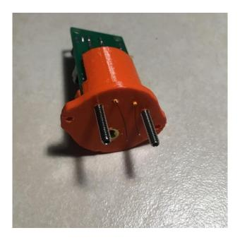
\_\_\_ For each post: Slide a #4 washer all the way down to the base of the main body. With a pair if needle nose pliers, wrap the wires clockwise snugly around the posts until there's no more left; it should be about two turns. Slide another #4 washer over the top of the wires, then screw a #4 nut finger-tight over the washer. Insert the .050" hex key wrench into the set screw, and with the pliers tighten the nut, holding the hex key wrench to prevent the set screw from rotating.
