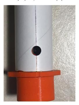
Using the mounting ring as a template, figure out where you're going to mount your Easy Mount. Remember that the screw switch must face the outside of your rocket, if you're using it... you can use the index mark in the mounting ring to locate it. The index mark needs to face the center of your body tube/coupler/payload tube/nose cone shoulder.
