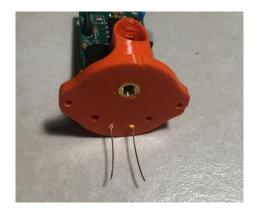
Using the .050" hex key wrench, screw the two #4 x  $\frac{3}{4}$ " set screws into the holes on the bottom of the main body, they should go in about  $\frac{1}{4}$ " so that about  $\frac{3}{4}$ " remains.
