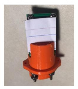
\_\_\_ Slide the battery into the slot in the mount. Bend the battery wire over the top-middle of the board, then insert the top cap over the Apogee board, and screw it on from the back side. Do not overtighten; finger-tight is fine.
