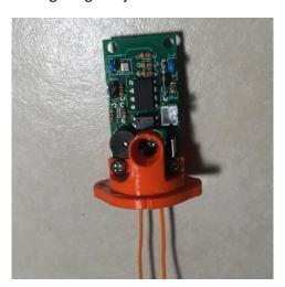
\_\_ Cut the two wires 1 ¼" from the bottom of the main body. Strip the insulation off the wires... you can use a wire stripper, or you can just use your fingernails and pull the insulation off. It's OK if there's a little stub of insulation at the bottom of the main body.
