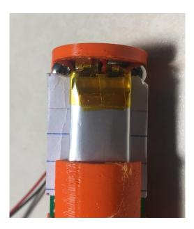
\_\_ Plug the battery connector into the JST-PH connector on the Apogee's board. Turn the screw switch on to confirm that it's beeping, then turn it off by backing out the screw one turn.
