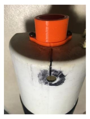
Prepare the 24mm motor mount tube by drawing a line down the center. Make a perpendicular mark ½" from the edge of the tube, then use a hole punch to punch out a hole centered on the mark. Push the motor mount tube over the Easy Mount so that the hole lines up with the screw switch. The tube helps keep the battery in place, and also helps protect the Apogee.
