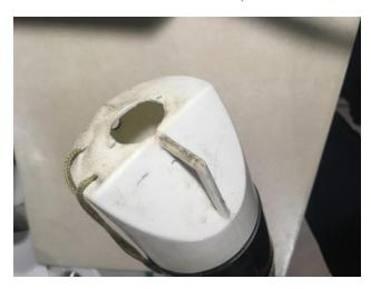
\_\_\_ Trial-fit the Easy Mount. Note that the screw hole must face the OUTSIDE of the nose cone shoulder. There is an index mark on the base of the Easy Mount which lines up with the screw switch, use that to make sure that the switch will be square with the nose cone shoulder. Drill two 1/16" pilot holes for the screws.
