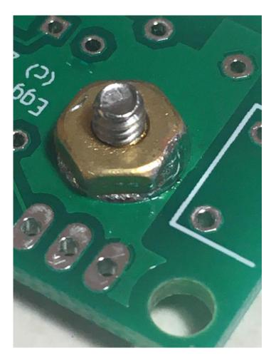
Once you're satisfied with the solder joint, allow the nut to cool for approximately 5 minutes, then turn the board over and back out the screw about two turns.
