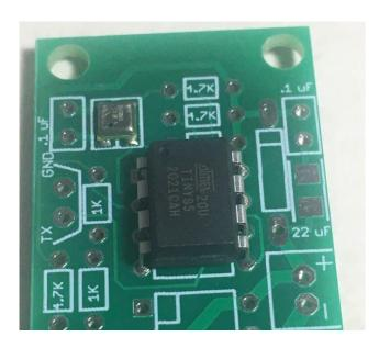
Locate the spot for the optoisolator, it's the 4-pin part just below the processor. Note that there is a notch marked on the silkscreen, this corresponds to the Pin-1 mark on the optoisolator chip. This MUST match with the "Pin 1" side of the optoisolatr. If you look at the optoisolator, you will see an indent, dot, triangle, or bar at one end of the package. That side is the one that must be matched up with the notch on the board.
