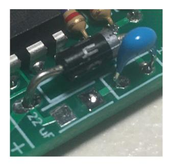
Holding the 22 uF capacitor with tweezers in one hand and the soldering iron in the other, gently heat up the tinned pad and place the capacitor onto the pads. Remove the iron, and wait about 5 seconds before letting go of the capacitor. If you've done it right, the capacitor should be soldered to that pad.
