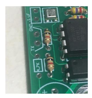
Locate the spot for the 4.7K resistor (yellow-purple-red) to the bottom-left of the optoisolator. Bend the leads close to the body, then insert them into the board. Use a piece of masking tape to hold them down, then turn the board over and solder the leads to the pads. Clip the leads off close to the board, then remove the masking tape.
