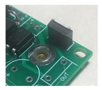
Locate the spot for the 22 uF capacitor, just to the right of the diode. This is a surface-mount part... there are no holes. The soldering technique is slightly different, but it's really no harder... it just "different".
