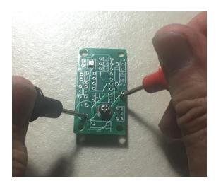
Now, close the screw firmly (but do not force it... don't use gorilla force!), then check the continuity between the "-" pad on the BATT connector and the pad on the buzzer that is not marked... you SHOULD now have continuity.
