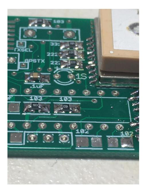
Locate the .1 uF capacitor just to the left of the resistors you just soldered, it will be marked .1 uF. Remove ONE .1 uF capacitor from the tape (it will be brown), and solder it in place. Inspect the solder joints with a 10x jeweler's loupe to make sure you don't have any solder bridges.
