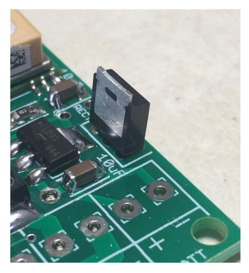
Insert the push button switch into the holes on the board. It has a little kink in the leads, so it will stand off about 1/16" if you have the kink centered in the middle of the hole. Turn over the board and solder the leads to the board.
