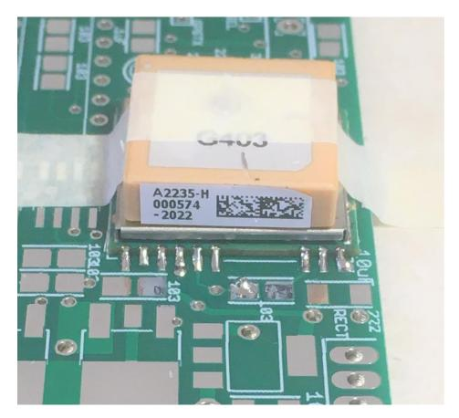
\_\_\_\_\_ Using as little solder as possible, solder the remaining pads on the GPS module, skipping pads and alternating sides so that you do not solder adjacent pads consecutively. This helps prevent the GPS module from getting too hot. Be sure to allow each solder joint to cool for at least 30 seconds before you move on to the next one.
