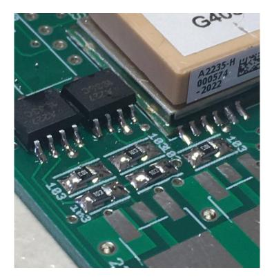
\_\_\_\_\_Before you go onto the next step, take this opportunity to look at the GPS pads on the right-hand side one more time with your 10x jeweler's loupe, to make sure that you have good solder joints that cover the pad AND the half-moon pads on the GPS module. Once you start soldering components next to the GPS module, it's going to be harder to get to it, so one more look right here may save you a lot of time later...
