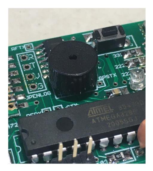
Assembly of your Eggtimer TRS is now complete. Inspect the board carefully, looking for "cold" solder joints or incomplete solder joints. Cold solder joints appear dull instead of shiny, and may appear as blobs of solder and not have the nice "wetting" of the pad that you will see with good joints. A magnifying light is good for checking the board. We do not recommend using flux remover or other cleaners on this board, as they may not be compatible with the no-clean flux in the solder.
