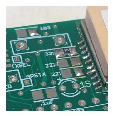
Locate the two 2.2K resistors just to the left of the GPS module and just below the 330 ohm resistor that you just mounted (it will be marked "222"). Remove two 2.2K resistors (marked "222") from the tape and solder it in place. Inspect the solder joints with a 10x jeweler's loupe to make sure you don't have any solder bridges.
