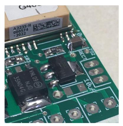
Locate the second 10 uF capacitor just to the left of the pads marked "BATT", it's marked "10 uF". Solder it into place, being careful to avoid solder bridges and inspecting it as you go.
