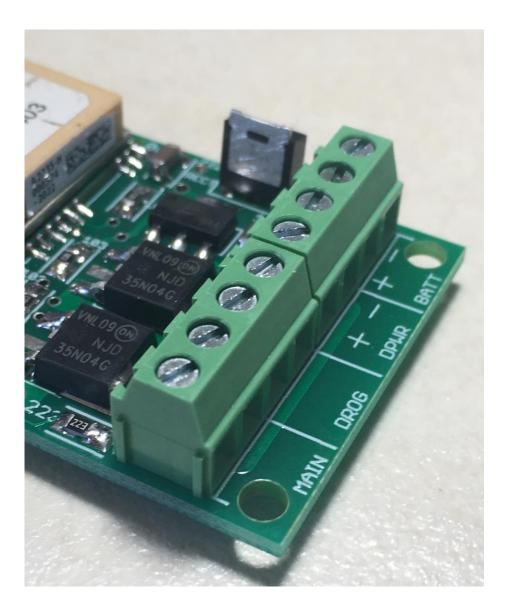
Strip about 1/8" from your battery connector wires, and tin the ends so they won't fray.
