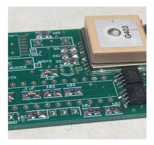
Locate the spot on the board for the SN74HC02 Quad NOR Gate, it's a SOIC-14 package (14 leads, surface mount with "J" leads). Using only a tiny bit of solder, tin the lower right pad on the PC board.
