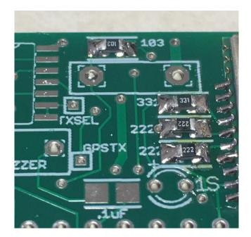
Locate the .1 uF capacitor about ½ inch below the resistors you just soldered, it will be marked .1 uF. It is just above the long row of pads for the processor, and is just to the left of the spot for the LED marked "1S". Remove ONE .1 uF capacitor from the tape (it will be brown), and solder it in place. Inspect the solder joints with a 10x jeweler's loupe to make sure you don't have any solder bridges.
