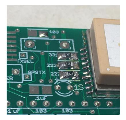
Locate the 10K resistor near the top of the board and to the left of the resistors that you just mounted (it will be marked "103"). Remove ONE 10K resistor (marked "103") from the tape and solder it in place. Inspect the solder joints with a 10x jeweler's loupe to make sure you don't have any solder bridges.
