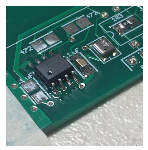
Locate the .1 uF capacitor just to the left of the EEPROM, it will be marked .1 uF. Remove ONE .1 uF capacitor from the tape (it will be brown), and solder it in place. Inspect the solder joints with a 10x jeweler's loupe to make sure you don't have any solder bridges.
