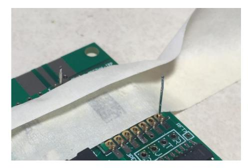
\_\_\_\_\_ Solder the BOTTOM LEFT pad of the Hope RF module to the board. Make sure that the board is properly positioned after you solder this joint; it it moves, heat up the solder joint and move the board slightly so that it is properly positioned. Wait 30 seconds after soldering before continuing.
