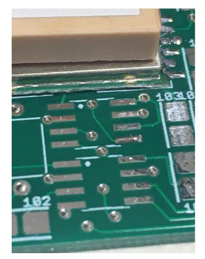
\_\_\_\_\_ Remove ONE of the ACPL-227 optoisolators from its carrier. With tweezers, gently place it onto the upper pads. If there is a notch on the optoisolator, it should be facing up. If not, the writing should be going from top to bottom (i.e. readable from the left side of the board).
