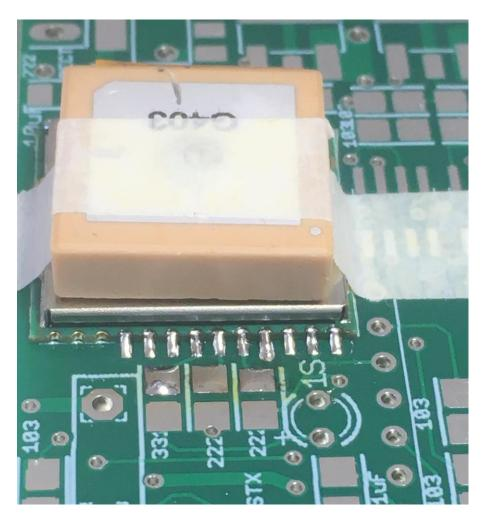
\_\_\_\_ Remove the masking tape from the GPS module, and remove the masking tape holding the board to your work surface. Turn the module over, and with two new pieces of masking tape tack it down to your work surface so it will not move (yes, it will be upside-down).
