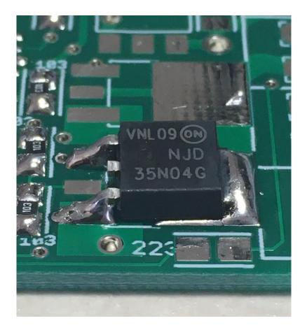
When you are done, inspect the solder joints to make sure that they are nice and shiny and that there are no solder bridges. Note: A solder bridge in an deployment transistor can cause a short that may destroy your Eggtimer TRS, and possibly your LiPo battery too. It may also possibly cause an unexpected deployment when you connect the battery. Be very careful here!
