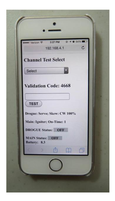
This is pretty explanatory... there's a pull-down to select the channel that you want to test, then you simply enter the 4-digit validation code and click on the TEST button. The channel settings are inherited from the Global Settings page... for example, if you have a channel set to be used in igniter mode with a 3-second firing time then that channel will fire for 3 seconds.
