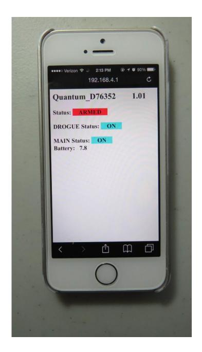
This page looks a lot like the status page, but the status is changed to "ARMED", it doesn't initially have the validation code/box, and only the channel continuity status and the battery voltage are displayed. A few seconds later you should start hearing the buzzer beep about once per second. This is an audible confirmation that the Quantum is now in flight sequence mode, and you're ready for launch.
