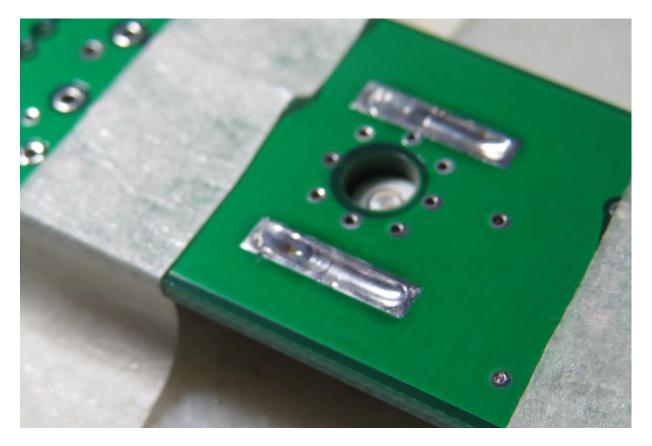
\_\_\_\_ Remove the masking tape from the board, turn it over so that the GPS module is now on top, and tape the board down to your work surface again.
