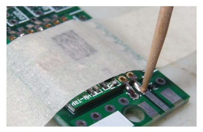
\_\_\_\_\_Solder the remaining pads to the board, waiting 30 seconds between pads to prevent the module from overheating. If you inserted leads into the holes to line them up, be sure to remove them before soldering.
