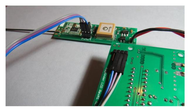
• Turn on the LCD receiver's power... the TX should also come on with BOTH the RED and GREEN LED's on the RF module lighting up. If it does NOT come on like this, immediately turn off the LCD's power and check your connections.
