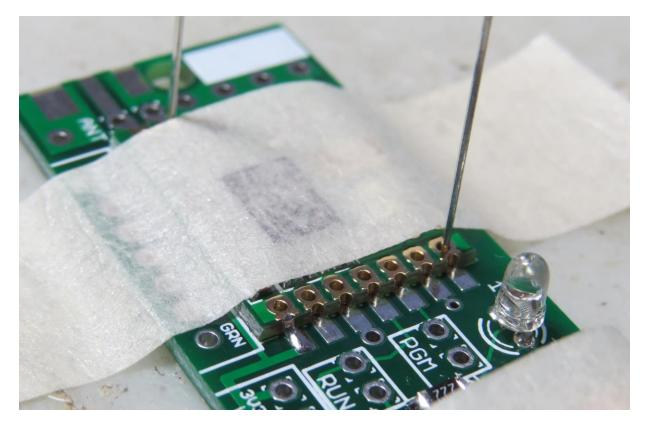
\_\_\_\_\_ Solder the pad on the left side that does NOT have the positioning lead in it. Be VERY careful not to create a solder bridge to the ANT pad!
