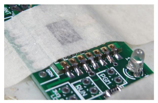
\_\_\_\_\_ If the TX came with a fixed frequency (not 915 MHz), with a permanent marker, write the RF module's frequency on the board in the space provided (i.e. "921"). Since the B and C revisions of the TX board can be frequency-programmed using the Eggfinder LCD you may not want to do this, but if you purchased a fixed-frequency receiver (such as the Eggfinder RX) then the frequency must match, so marking it would be prudent.
