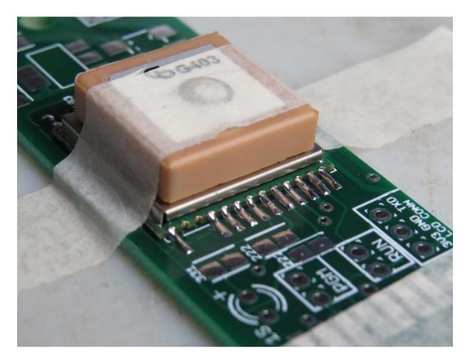
Using as little solder as possible, solder the remaining pads on the GPS module, skipping pads and alternating sides so that you do not solder adjacent pads consecutively. This helps prevent the GPS module from getting too hot. Be sure to allow each solder joint to cool for at least 30 seconds before you move on to the next one. Make sure that the solder joints fill the "half moon" cutouts in the GPS module pads.
