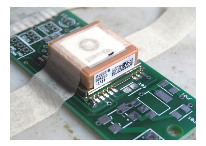
\_\_\_\_\_CHECK AGAIN that the GPS module is properly oriented and that the pads are centered on the PC board's pads. If the GPS module moved a little during soldering, heat up the solder joint and GENTLY move it into place. If you cannot get it to move without removing it, remove the masking tape, heat up the solder joint, then GENTLY lift the module from the board. Remove the solder with some wick, get a new piece of masking tape, and try again.
