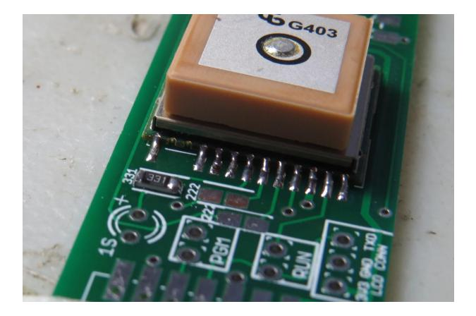
\_\_\_\_ Mount the 2.2K Resistors (marked "222" or "2211")
