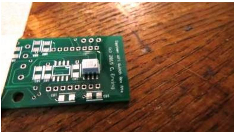
When you're done, solder the right optoisolator in place using the same procedure. Inspect the joints carefully... the optoisolators have short stubby leads, and it's relatively easy to have the solder on the pads miss the leads if you don't use enough solder.
