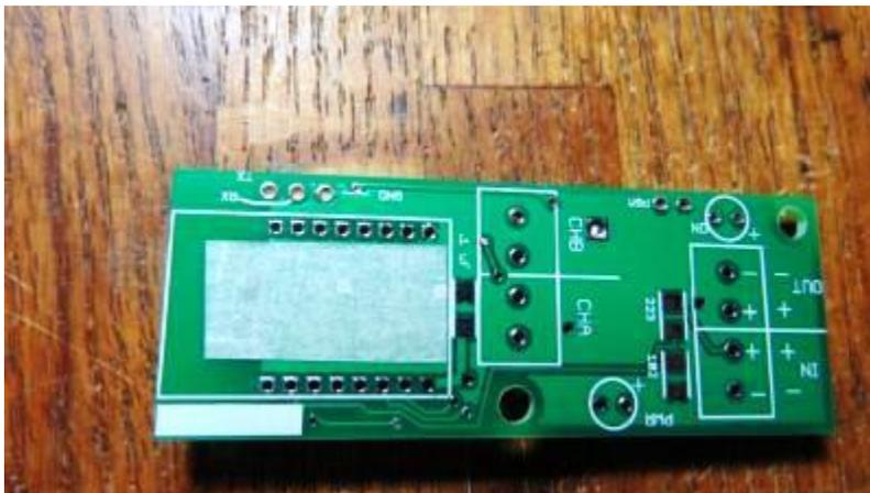
Turn the PC board over so that the BOTTOM side (the one with the optoisolators, etc.) is “up”. Prop the board up so that there’s about 1/8” or so underneath the board. Take one of the 1/8W resistors and put it into one of the corner holes where the WiFi modules pads are.. Yes, it will stick up a lot. Solder the lead to the pad, then clip the lead off at the pad. Insert the resistor’s leads into the next three corners, soldering them to the pads.
