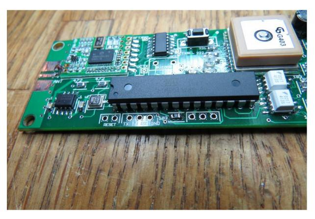
Locate the spot for the resonator, it's 3 pads at the bottom of the board right in the middle of the processor, marked "XTAL". Place the resonator in its place, tape it down so it won't fall out, turn the board over and solder the pins. Trim the leads flush.
