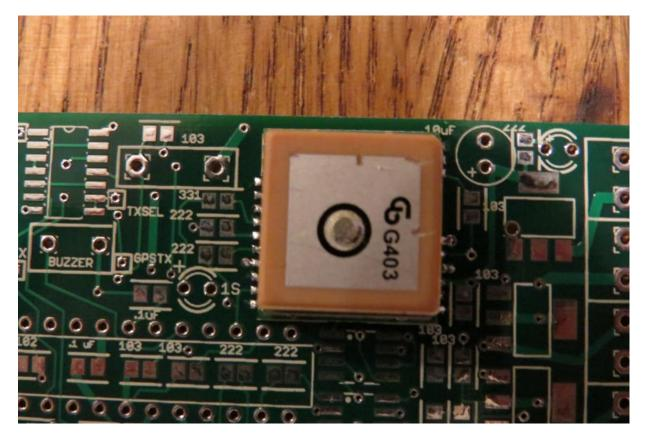
Remove the masking tape from the GPS module, and remove the masking tape holding the board to your work surface. Turn the module over, and with two new pieces of masking tape tack it down to your work surface so it will not move (yes, it will be upside-down).
