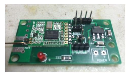
If you are building the Bluetooth version with the case, they will be mounted on the BOTTOM side of the board, opposite the other parts. This is because the board will be mounted in the case with the RF module facing out, so the headers need to face inwards so they're accessible once the board is mounted.
