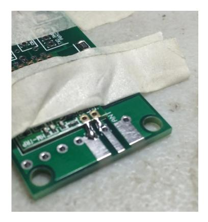
\_\_\_ Solder the remaining pads to the board, waiting 30 seconds between pads to prevent the module from overheating. (If you put a positioning wire in that pad, remove it before soldering).
