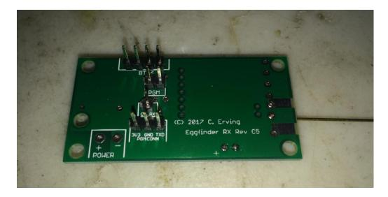
Insert the headers into the appropriate pads, we recommend that you use some masking tape to hold them in place. Turn the board over and solder all the pins. Don't oversolder... you only need enough to ensure that there's a good connection.
