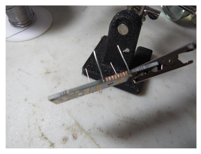
\_\_\_ Gently set the board down on the table. Place the GPS module on the board so that the pads align with the four resistors. Note that on one cornet the wires are not at the end of the GPS module, they're four pads inwards. If you did it right, the GPS module's half-mood pads will be in perfect alignment will all of the channels on the PC board. You may need to squeeze the leads in slightly to get a good fit.
