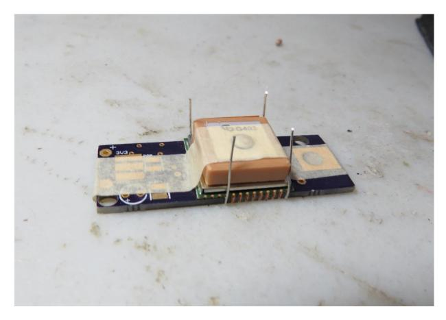
\_\_ Cut a piece of paper masking tape about 3/8" wide and 2" long, and carefully tape the GPS module down to the PC board. Make sure it's a nice snug fit, you don't want the GPS module coming loose in the next step.
