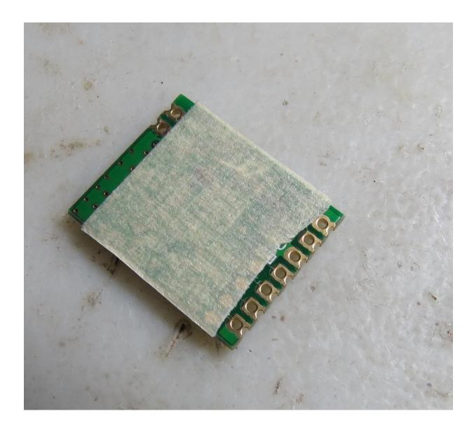
Carefully position the Hope RF module on the board so that its pads line up in the center of the top pads, the "half-moon" cutouts on the module should be centered on the pads on the board. Make sure that it's properly positioned, there are some small holes on the pads on the module, they should line up with similar holes on the board. Use the cut-off LED leads to line up the module, put one in each corner to line it up (you won't be soldering them in, they're just for alignment).
