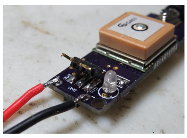
Solder your battery connector to the two pads near the edge of the board marked "+" and "-". Make sure that there are no stray wire "whiskers" touching the board.
