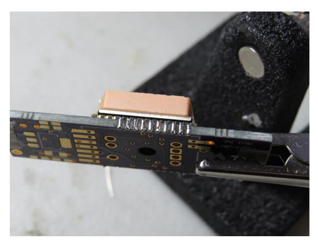
\_\_\_\_ After all of the open channels have been soldered, gently heat up one of the resistor leads and remove it, then fill up the channel and GPS pad that was there. Similarly, remove the other resistor lead, and fill up that channel. Be sure to use enough heat so that the leads want to fall off the board... if you don't, you might lift the pads along with the leads!
