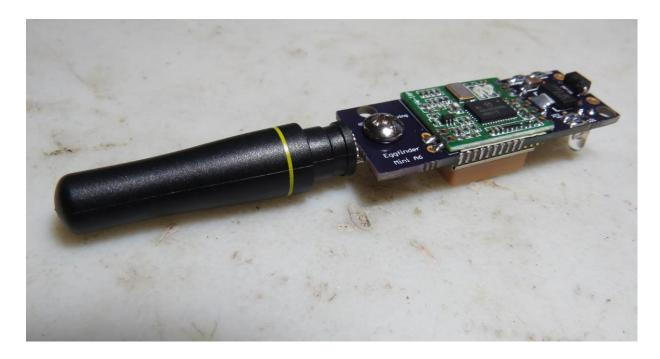
Assembly of your Eggfinder Mini is now complete. Inspect the board carefully, looking for "cold" solder joints or incomplete solder joints. Cold solder joints appear dull instead of shiny, and may appear as blobs of solder and not have the nice "wetting" of the pad that you will see with good joints. A magnifying light is good for checking the board. We do not recommend using flux remover or other cleaners on this board, as they may not be compatible with the noclean flux in the solder.
