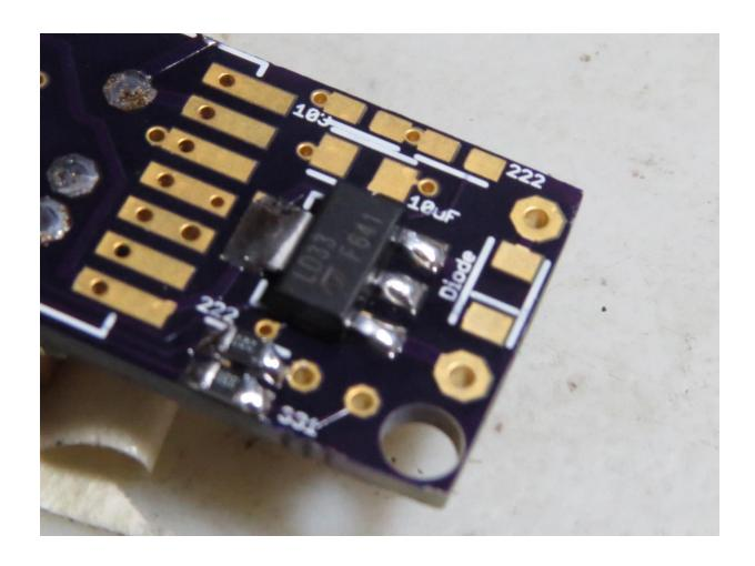
\_\_\_\_ Mount the 10 uF capacitor
