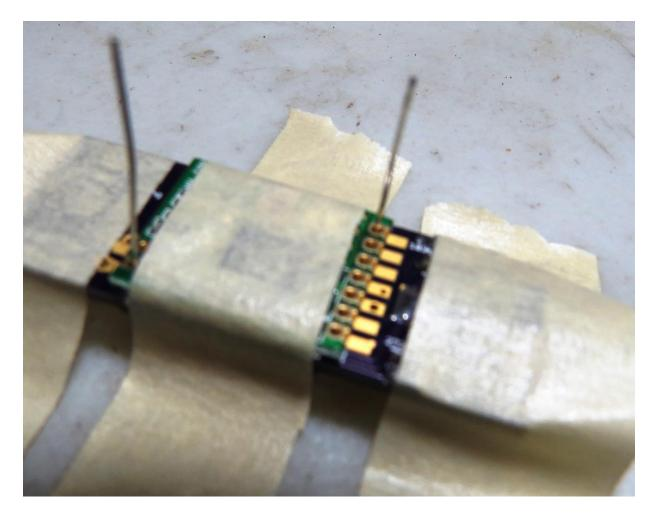
\_\_\_\_ Solder the second pad from the top-right of the Hope RF module to the board (the one NEXT to the positioning lead). Make sure that the board is properly positioned after you solder this joint; it it moves, heat up the solder joint and move the board slightly so that it is properly positioned. Wait 30 seconds after soldering before continuing.
