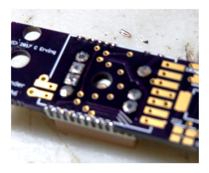
Inspect all GPS module solder joints to make sure that they are nice and shiny, and that they properly bridge the GPS module pads and the PC board pads. Leave the board taped down to your work surface for now (GPS side down).
