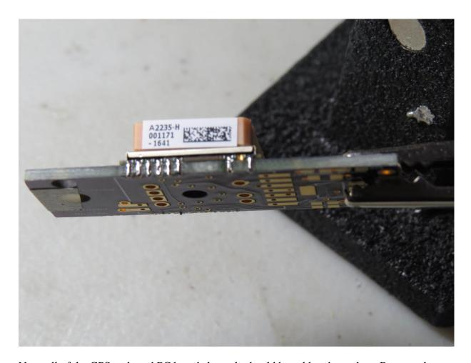
Now, all of the GPS pads and PC board channels should be soldered together. Remove the masking tape, and turn the board over on your table (yes, it will be upside-down).
