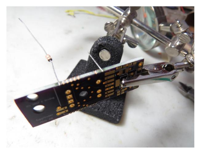
\_\_ Unclamp the board and turn it around so the other side with the half-moon pads is facing up. Tin the two channels at the ends, and solder resistor leads in them just as you did with the other end. Unclamp the board.
