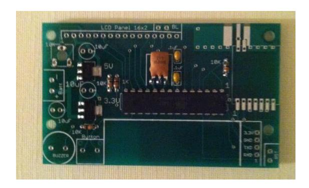
\_\_\_ Mount the 10 uF electrolytic capacitors
