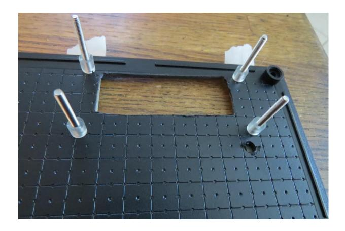
Now, carefully slide the Eggfinder board onto screws, and firmly press the 16-pin header socket on the Eggfinder board into the LCD panel's header. If everything was cut and positioned properly, the board should rest nicely on the pieces of tubing.
