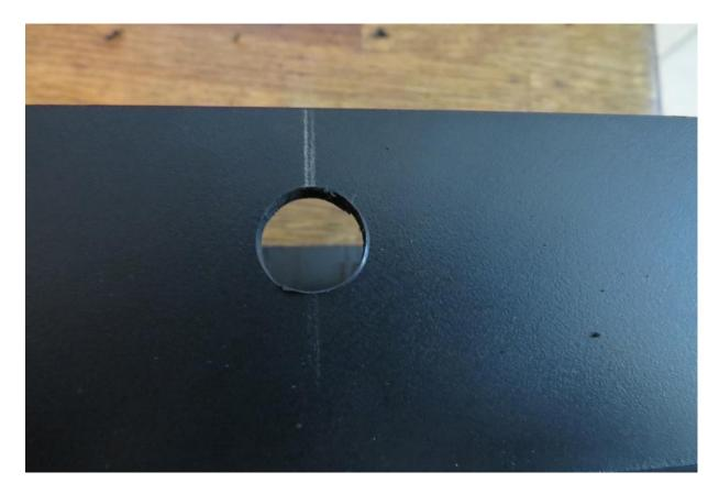
Now you need to drill a hole for the battery box switch. Drill a pilot hole in the bottom of the case bottom, 1" from the left edge and 1" from the bottom edge. Drill it out to ½" with a spade bit.
