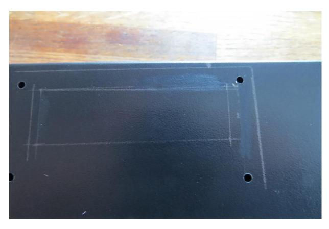
With a 1/8" drill bit, drill out the four mounting holes. Cut a 1/4" sound hole 5/16" below and 1/8" to the right of the bottom-left mounting hole.
