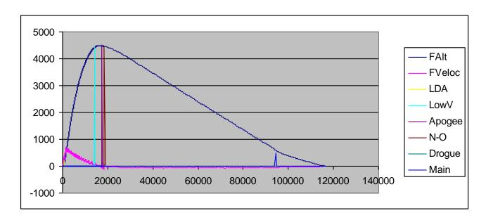
The "FAlt" trace is altitude @ time, the "FVeloc" trace is the filtered altitude @ time. The other "spikes" are event markers; they point to the altitude and time at which specific events in the flight have occurred. For example, the "LowV" marker shows that the Low Velocity event (the end of Mach Lockout, after 1 second of <100 ft/sec velocity has been detected) occurred at about 17 seconds and 4400 feet.
