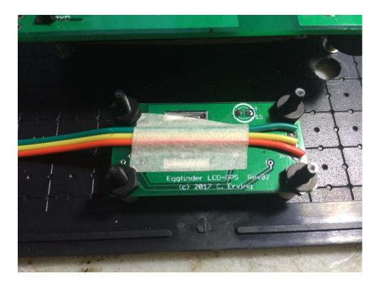
\_\_\_\_\_ Carefully remove the tape from the LCD-GPS board. Lift the cable up a little, and with a hot melt glue gun put a blob of glue just to the left of the cable pads. Lay the cable down onto the glue, and let it cool for a few minutes. The idea is to allow you to move the cable without disturbing the relatively fragile wires soldered to the pads.
