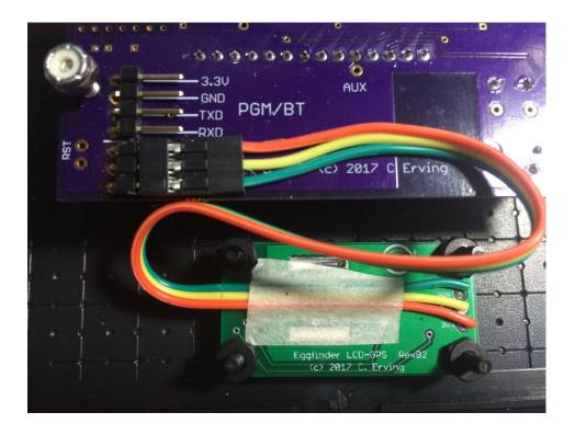
Assembly of your Eggfinder TX is now complete. Inspect the board carefully, looking for "cold" solder joints or incomplete solder joints. Cold solder joints appear dull instead of shiny, and may appear as blobs of solder and not have the nice "wetting" of the pad that you will see with good joints. A magnifying light is good for checking the board. We do not recommend using flux remover or other cleaners on this board, as they may not be compatible with the no-clean flux in the solder.
